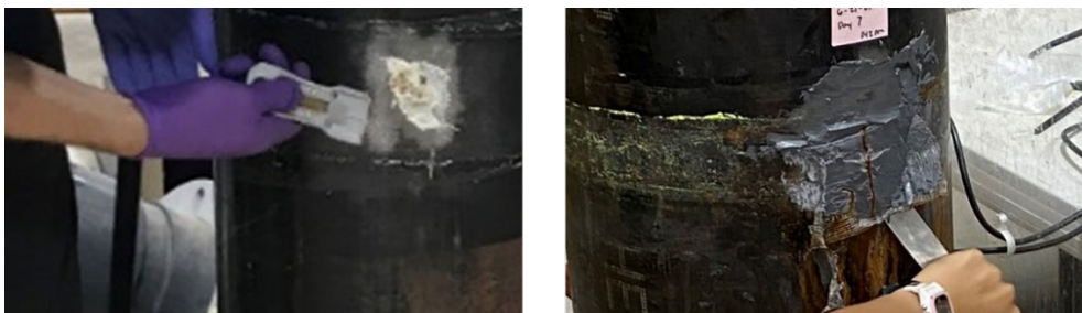
Figure 8.—Removing repair product from pressure vessels after testing is complete. Left: using a scraper knife. Right: using a chisel and mallet.
