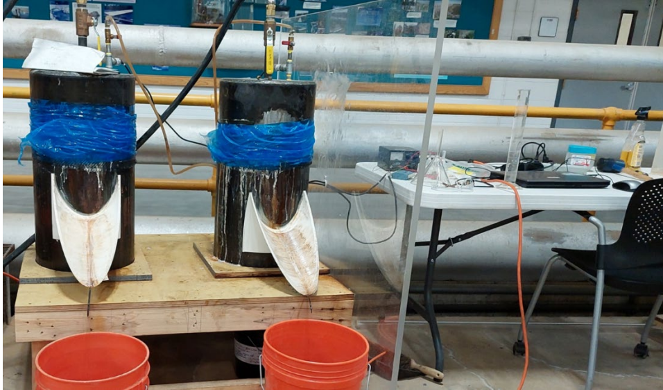
Figure 7.—Laboratory testing set-up showing two pressure vessels with plastic spouts to direct water leakage into the measurement buckets below. The power supply, DAQ device, and laptop are set up on a table on the right side, with a plexiglass pane to protect the equipment from any spraying water.
