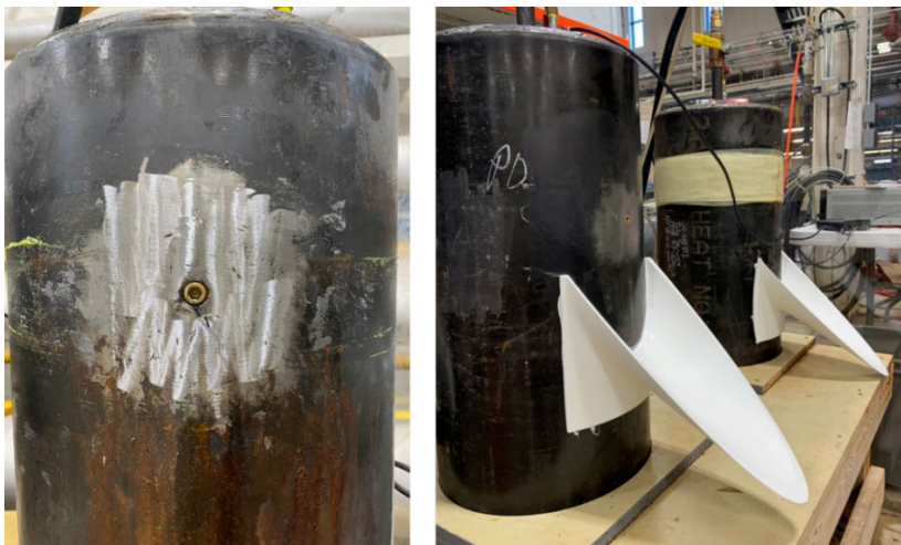
Figure 2.—Left: brass plug inserted in pressure vessel to simulate leak. Right: two pressure vessels, each with a 3D-printed spout to direct water leakage.
