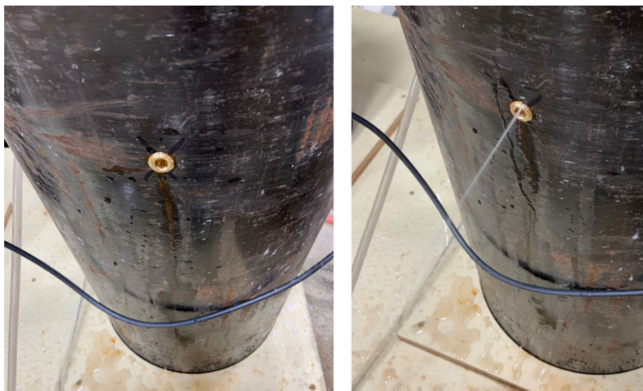
Figure 4.—Brass plugs providing different leak conditions. Left: weeping leak with water running down the surface of the pressure vessel. Right: spraying leak with water shooting out from the plug.
