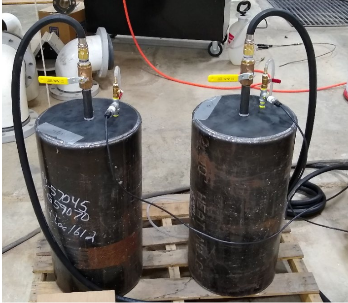
Figure 1.—Pressure vessels after pressure testing.
